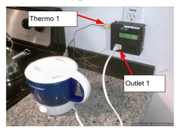
3) Position the thermocouple so that the tip sits near the middle of the water
