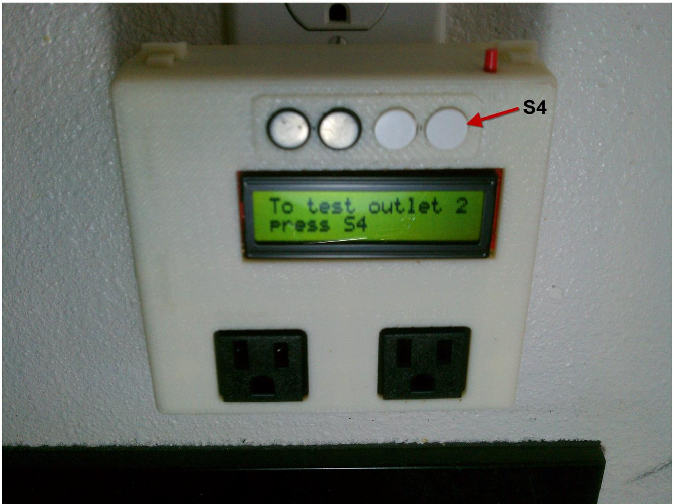
Use S1 to toggle the relay for Outlet 2 and confirm that there is a clicking sound. When you are ready to move on press S2
