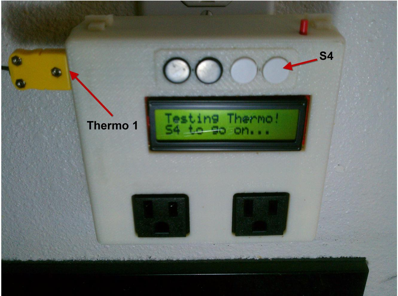
Wait for the temperature reading to settle. If you've just plugged the thermocouple in this could take a few seconds. Now is the time to verify that the number is within the realm of reason. The testing software is setup to give an approximate Farenheit scale reading.
