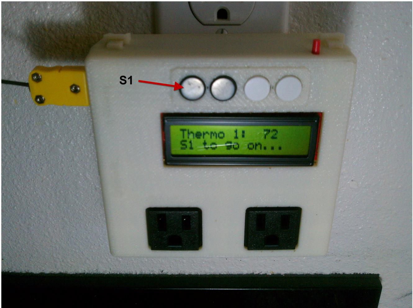
Plug the thermocouple into Thermo 2 and wait for the number to settle. Then again satisfy yourself that Thermo 2 is working approximately correctly.
