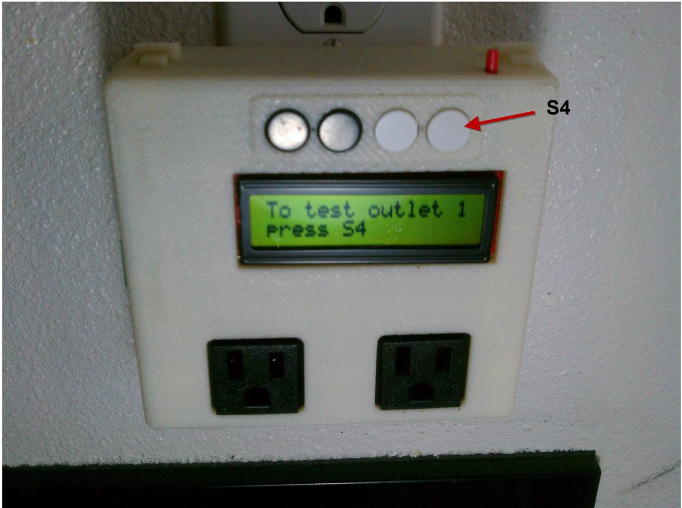
Both outlets are controlled by mechanical relays. Thus when they are activated (turned on) there is an audible “click” sound. Likewise when the relay is deactivated, there is another audible click as the mechanical components go back to their original position.
