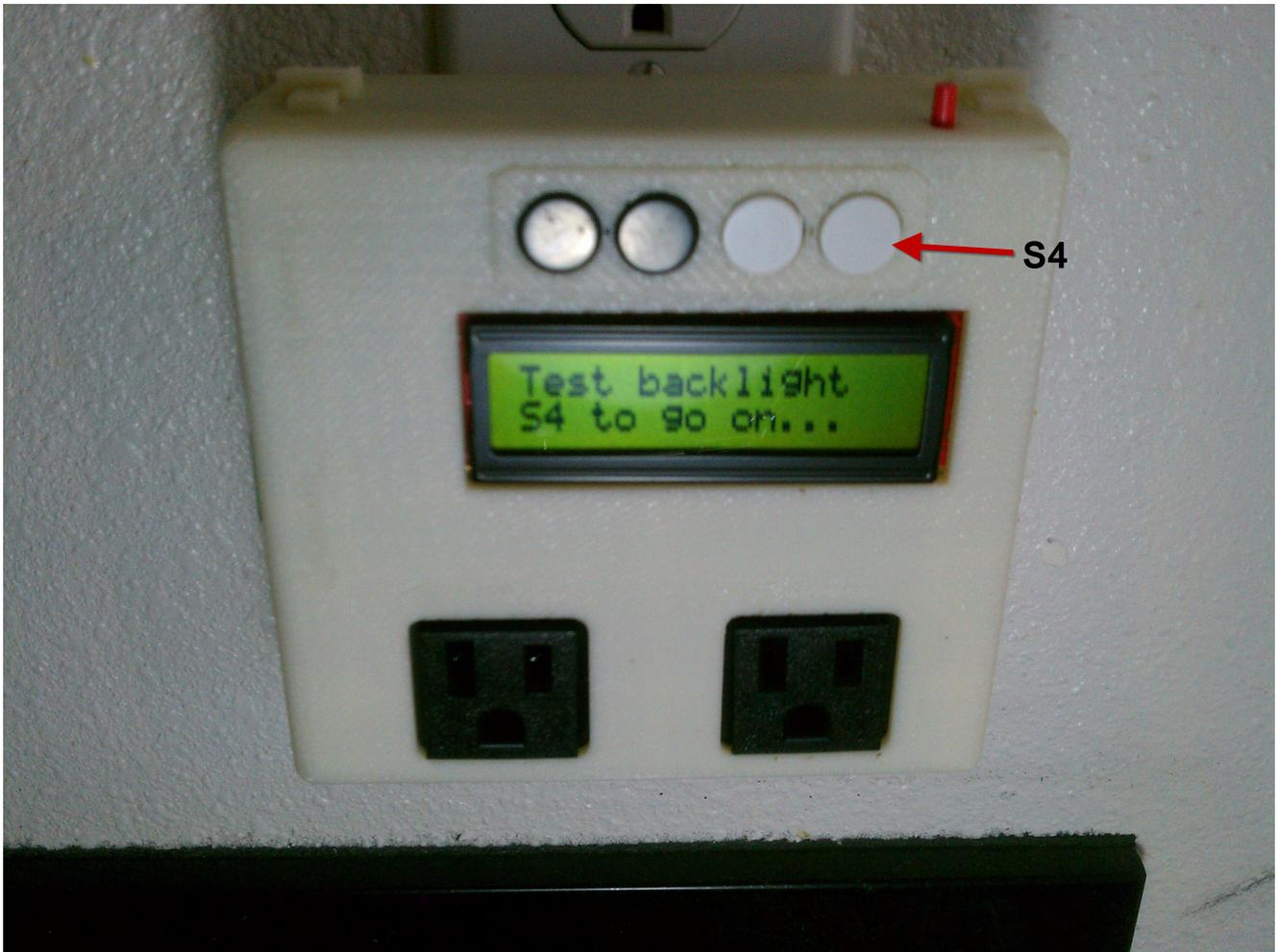
With everything working correctly, the backlight will turn on while S1 is pressed and then will turn off when S1 is released. Once satisfied that it is working, press S2 to continue.
