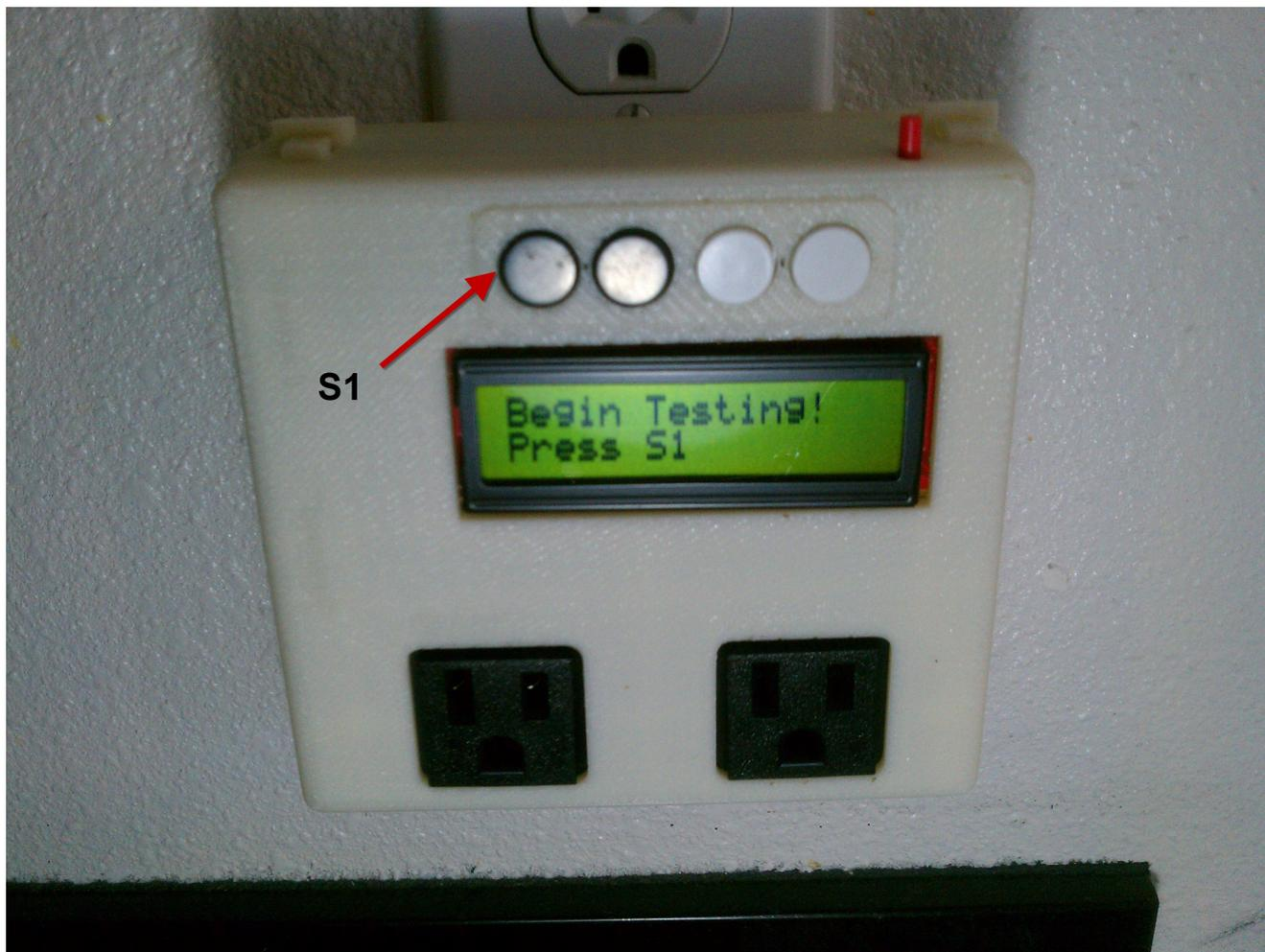
Next is a series of screens to make sure each button is working correctly. As you push each of the buttons S1, S2, S3, and S4 the screen confirms that the button works and asks that you press the next button in the sequence.
